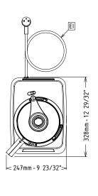
Electric **Supply voltage:** 220-240 V/1N ph/50 Hz Electrical power, max: 0.5 kW 0.5 kW **Total Watts:** Capacity: Performance (up to): 0 kg/Cycle Capacity: 2.6 litres Key Information: External dimensions, Width: 247 mm External dimensions, Depth: 328 mm External dimensions, Height: 456 mm **Shipping weight:** 15.2 kg Meat mincing capacity: 0 kg Mayonnaise preparation 0 kg capacity:
